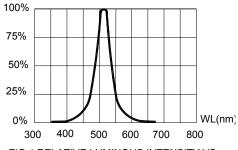
FIG.4 RELATIVE LUMINOUS INTENSITY VS. WAVELENGTH.
